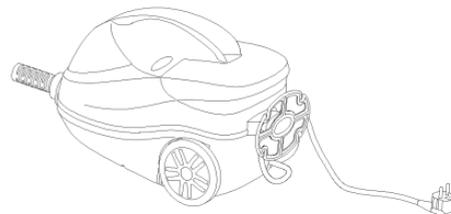
You can install the cord retractor on the back of unit and assemble the power cord on it.
